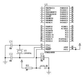
Fig. 2. ATMega8535 system minimum schematic.
