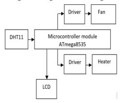
Fig. 1. System block diagram
