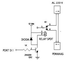
Fig. 4. Heater circuit schematic diagram.
