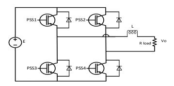
Fig 2. Topology full-bridge inverter
