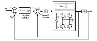
Fig. 3. Double-loop control system
