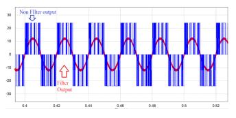
Fig 12. Result of simulation Non-filter output and Filtering output
