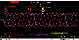
Fig 17. Result of implementation output voltage inverter TPFW double loop
