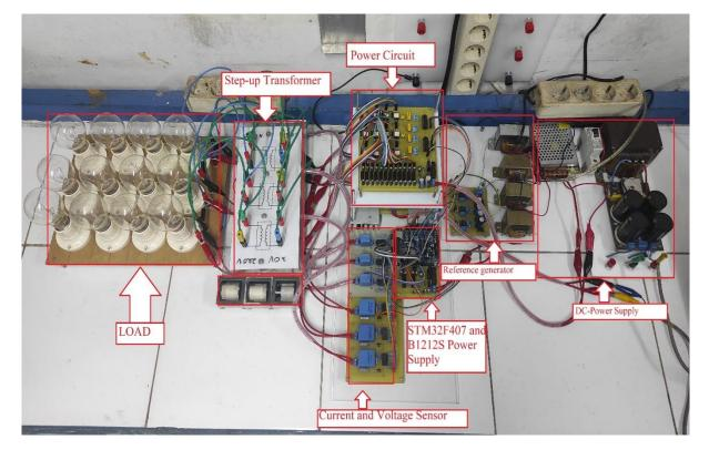
Fig 9. Hardware implementation double loop TPFW-Inverter
