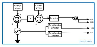
Fig. 7, Power circuit along with inverter three-phase four-wired control circuit
