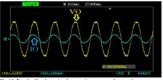
Fig 15. Result of hardware implementation output voltage and output current
