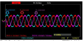
Fig 19. Result of implementation output current inverter TPFW double loop
