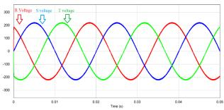
Fig 16. Result of simulation output voltage inverter TPFW double loop
