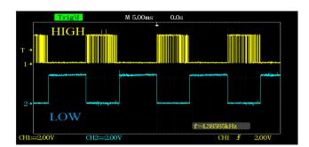
Fig 11. Switching hardware results in PWM from inverter TPFW
