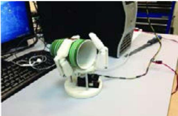
Figure 1. Two designs of three fingered adaptive underactuated end effectors.
