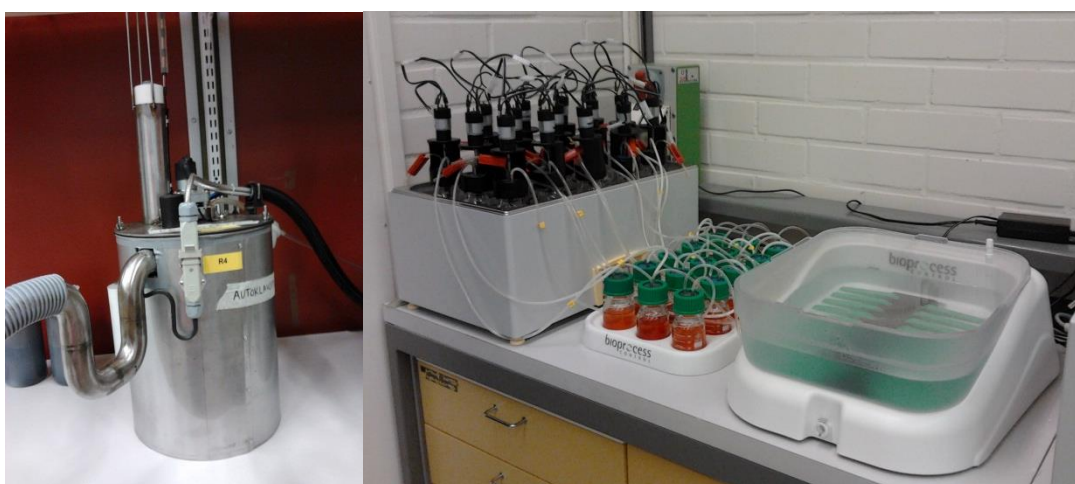
Figure 7. The laboratory stirred tank reactors (left) and BMP devices (right) used in this study.
