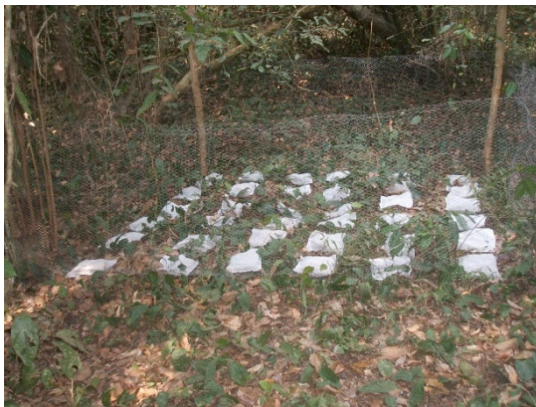
Figure 1: Litterbags exposure in the field
