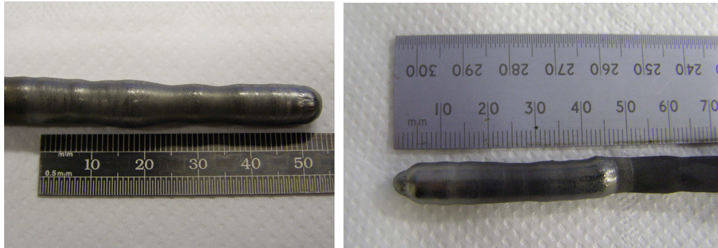
Figure 5.1: As-grown boules of Y_{0.15}Sr_{0.85}CoO_{3-\delta} (left panel) and Y_{0.2}Sr_{0.8}CoO_{3-\delta} (right panel) grown at speeds of 0.5-1 mm/hr using the floating-zone method.
