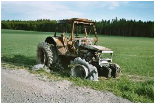
Figure 2. A tractor fire incident may include safety risks, production and economic losses and environmental risks (Photo: Jarkko Leppälä).
