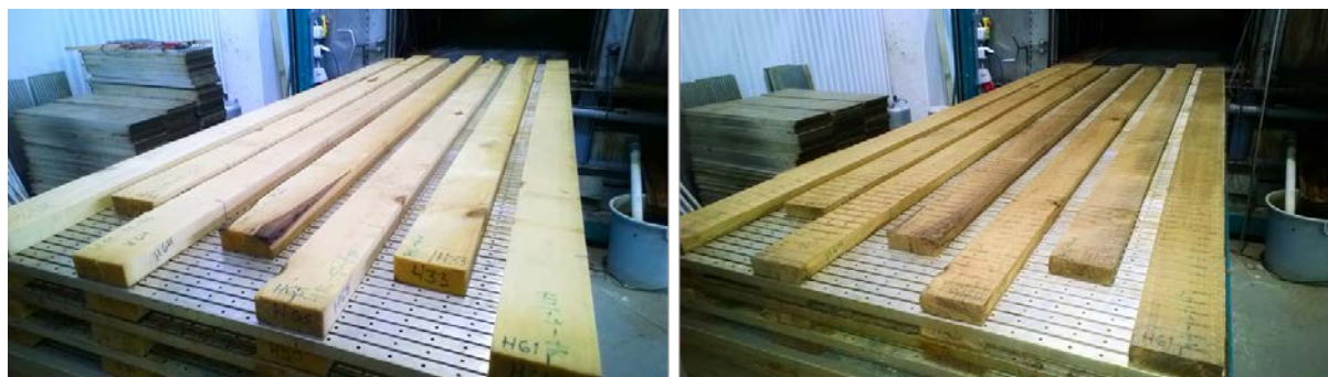
Fig. 1. A set of aspen boards (40x100x2700mm) before and after the compression and thermal modification process started at green state. Photos: Korwensuun Konetehdas Ltd.
