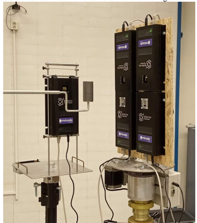
Fig. 3. Fast neutron calibration setup with an ^{241}\text{AmBe} source and five detectors operated simultaneously.
