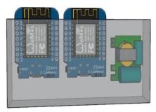
Fig. 4. Mesh gateway and MQTT gateway
