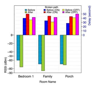
Fig 14. Switch ON/OFF testing for all light nodes when two disconnected light nodes
