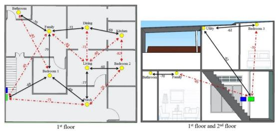
Fig. 12. Path of the gateway signal to all light nodes in the ESP-Mesh network
