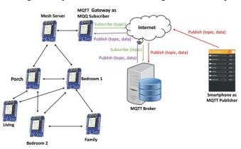
Fig 6. Working as an MQTT broker in the smart light system
