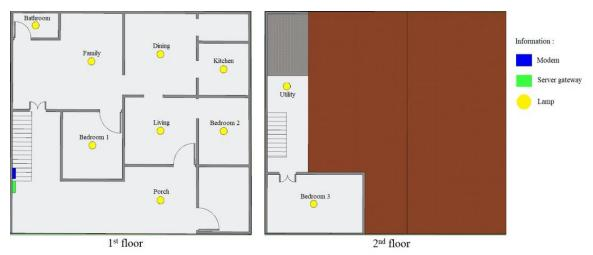
Fig. 9. The layout of the lamp placement
