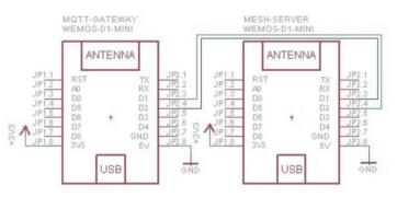
Fig. 5. Schematic of gateway circuit
