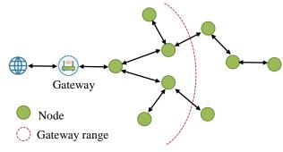
Fig. 1. Multi-hop ESP-Mesh network topology
