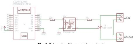
Fig. 3. Schematic of the smart lamp circuit
