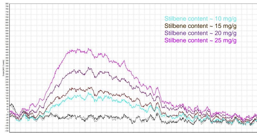
The higher the stilbene concentration is, the brighter is the blue colour, and the higher is the measured peak of fluorescence.
