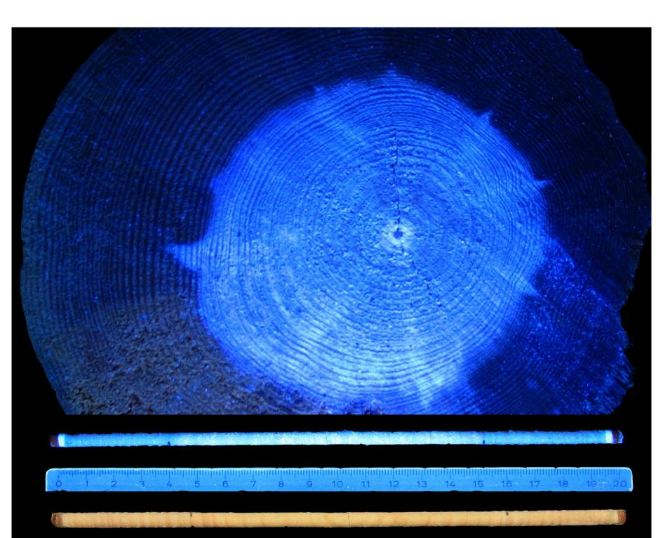
Under UV-light, stilbene-containing wood emits light blue colour, the intensity of which could be measured.
