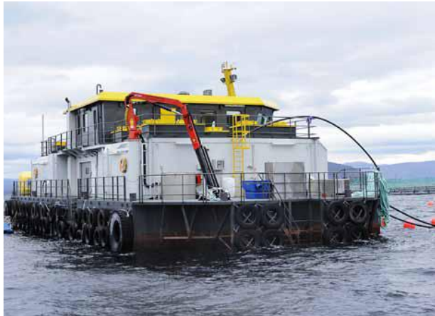
Figure 3 State of the art feed barges include feed silos, feeding system, monitoring centre, employee facilities and power devices
