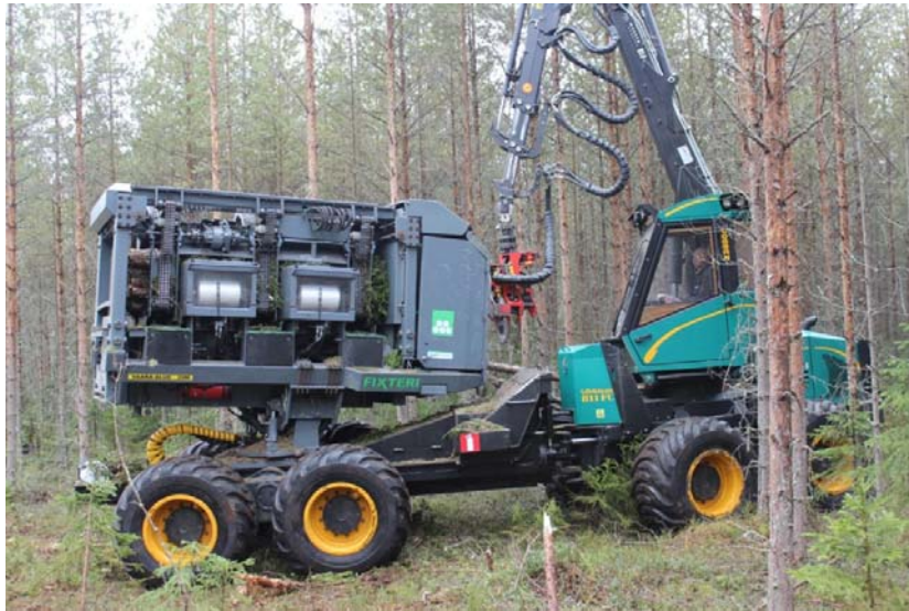
Figure 1. The Fixteri FX15 bundle-harvester system
