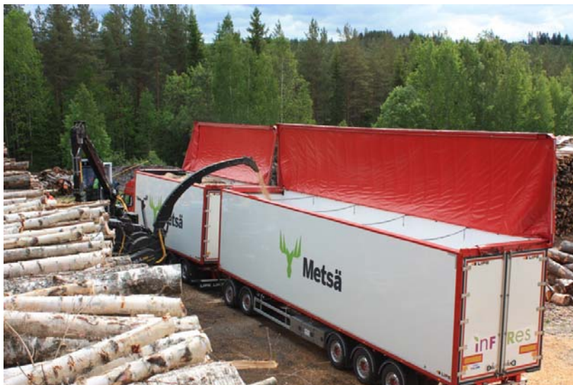
Figure 3 – The nine axle Lipe truck-trailer unit at the Tikkakoski roundwood terminal during the chipping/loading experiment (Photos: Petri Kaksonen/Kesla).
