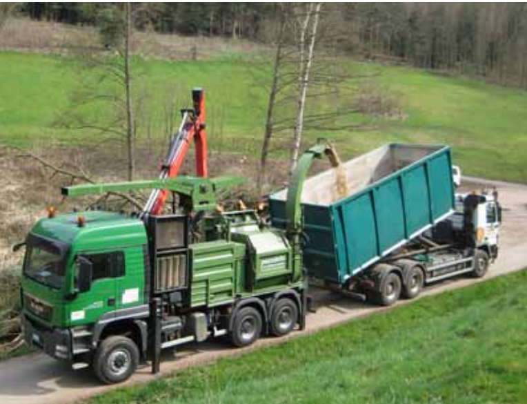
Innovative supply chain was demonstrated based on a new chipper-truck by Pezzolato, which is characterized by high power and compact design.
