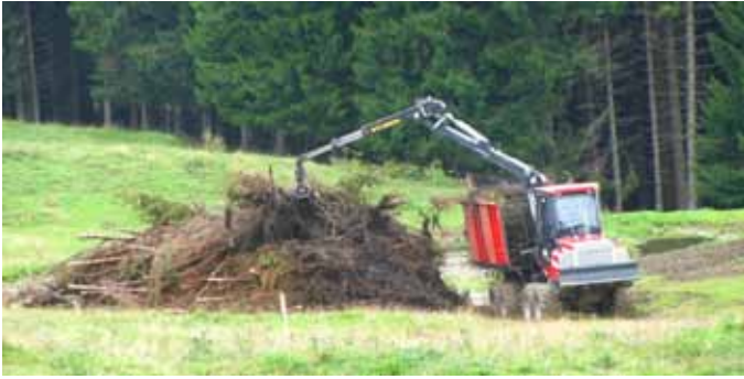
The new high-speed forwarder loading residues in its biomass cradle.
