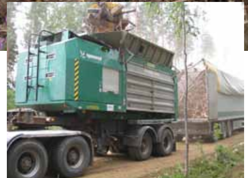
The Crambo crusher at work in Finland.
