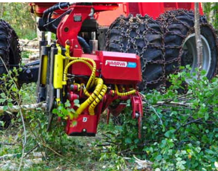
Multi-tree felling head Naarva Grip , which was demonstrated in Spain and Austria. Photo from Austrian demonstration.
