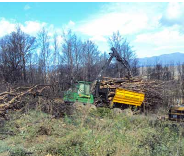
Press collector was demonstrated in Catalonia, Spain. The collector has a capacity of 40–48 m 3 .
