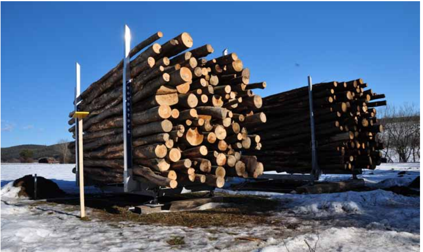
Metal frames on load cells, working like bygone large, permanent scale, are the state-of-the-art technology in monitoring wood fuel drying performance. Load data gained this way can be linked to meteorological data so as to develop wood fuel drying models.
