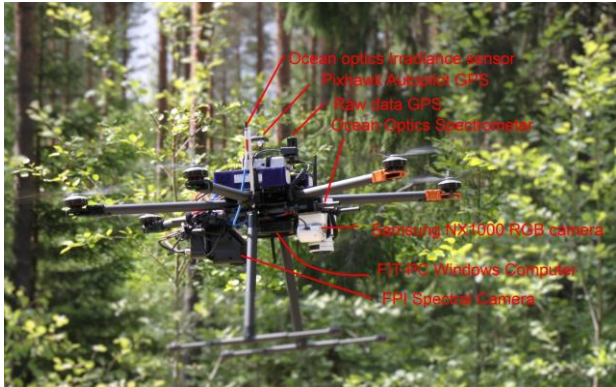
Figure 1. UAV imaging system.
