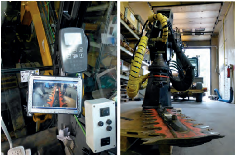
Figure 5. The operator-assisting camera system, equipped with a wide field-of-view Full-HD camera system installed on an excavator instrumented for forest management operations with a Mense clearing tool.
