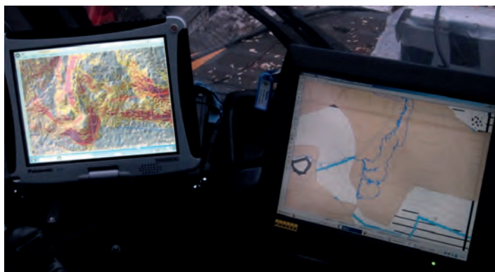
Figure 16. Enhanced terrain data of the Logging Map concept (left) alongside a traditional base map view (Photo: Metla/Jari Ala-Ilomäki).
