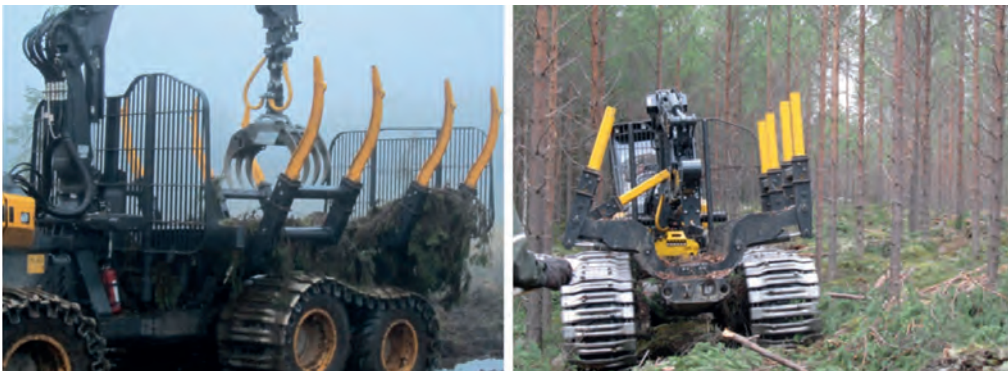
Figure 15. Left: Compressible load space for forwarding slash. Right: Compressible load space equipped with straight stakes suitable for roundwood forwarding as well as biomass compression.
