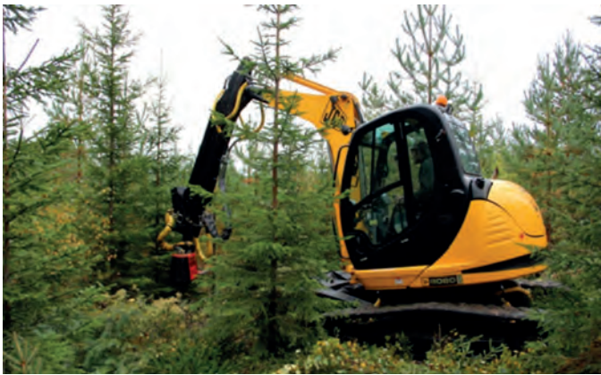
Figure 3. Risumoto machine equipped with Marttiini extension crane and Mense Rp40-clearing head.
