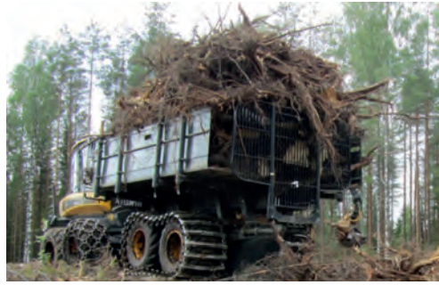
Figure 14. Extendible-width load space for stumpwood forwarding.
