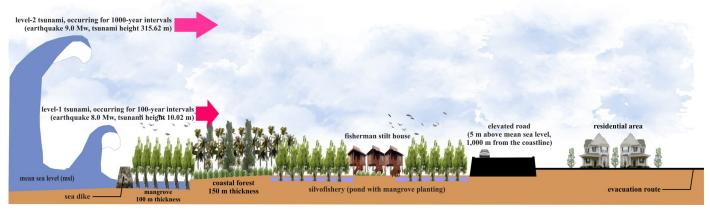
Figure 6. Conceptual Illustration of A Section of A New Approach of Tsunami Mitigation Strategies to Reduce The Risk of Tsunami Disasters and To Optimize The resources Through The Multi-Layer Defence Systems
