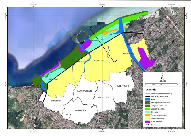
Figure 5. Conceptual Illustration of A New Approach of Tsunami Mitigation Strategies to Reduce The Risk of Tsunami Disasters and to Optimize The Resources Through The Multi-Layer Defence Systems
