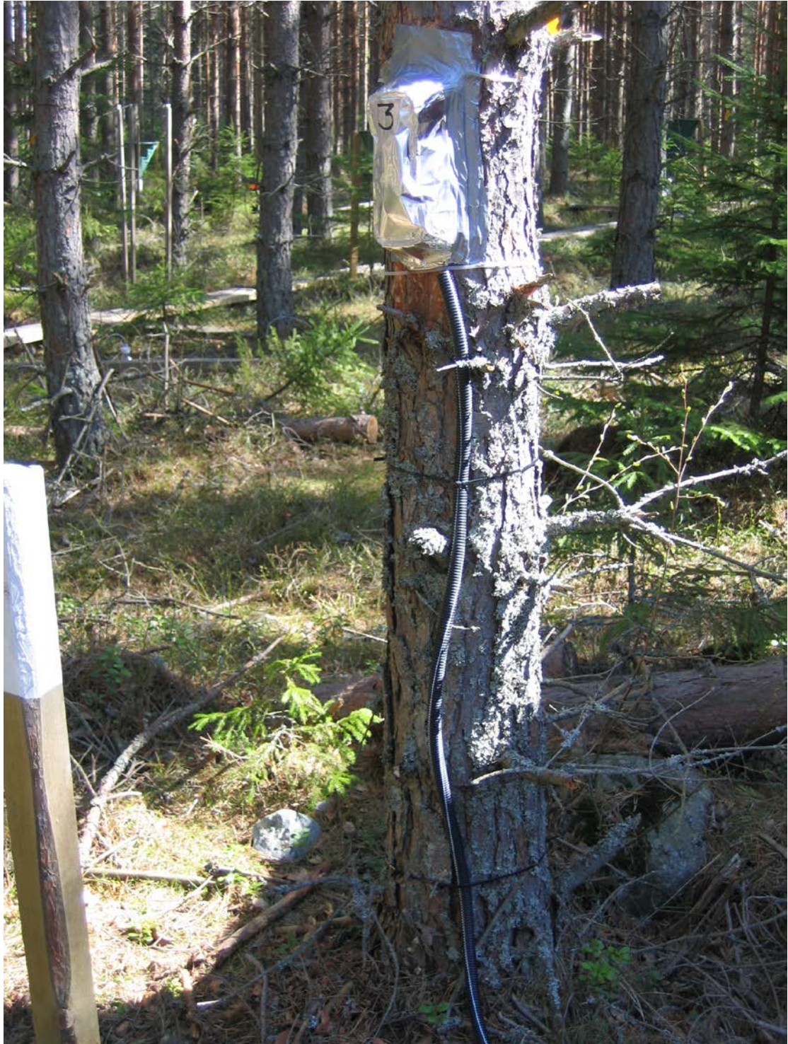
Figure 1. Sap flow sample tree with radiation shield installed over sensor pair.
