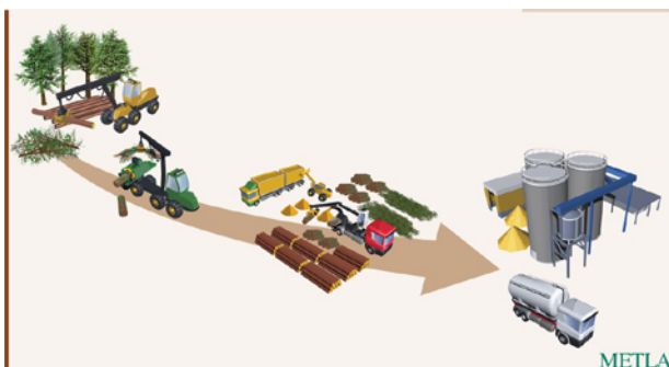
Figure 7. Bundling of logging residues after clear-felling with chipping at a terminal.
