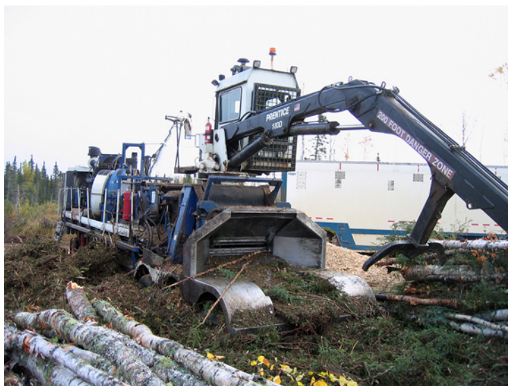
Figure 29. Whole tree chippers are delimiting, debarking and finally chipping the material. High qualities with low bark contents can be produced for high quality pulp and pellet production. © Dominik Röser, Metla.
