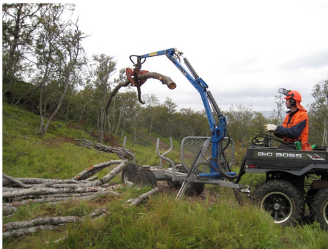
Figure 9. Small scale forwarding with ATV after motor manual fellings in Iceland. © Robert Prinz
