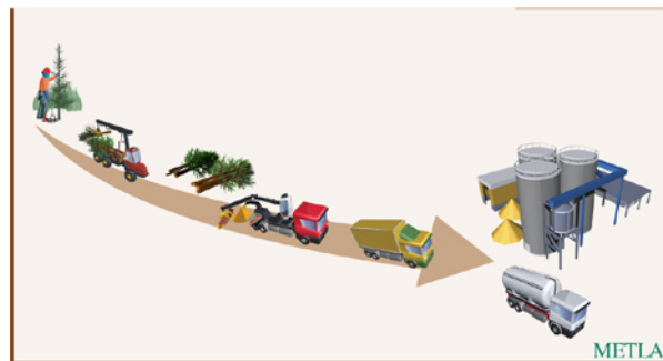
Figure 8. Manual harvesting of whole trees, roadside chipping and delivery of chips from the roadside to the pellet plant.
