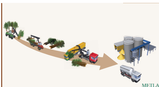
Figure 11. Mechanized harvesting of whole trees, roadside chipping and delivery of chips from the roadside to the pellet plant.
