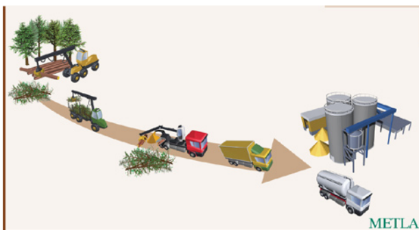
Figure 6. Collection of logging residues after clear-felling, roadside chipping and delivery of chips from the roadside to the pellet plant.
