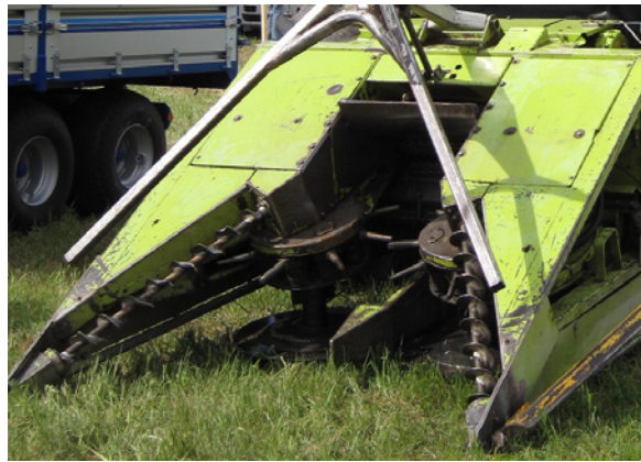
Figure 13. Claas Jaguar 850 field chipper with HS-2 cutting head. © Robert Prinz
