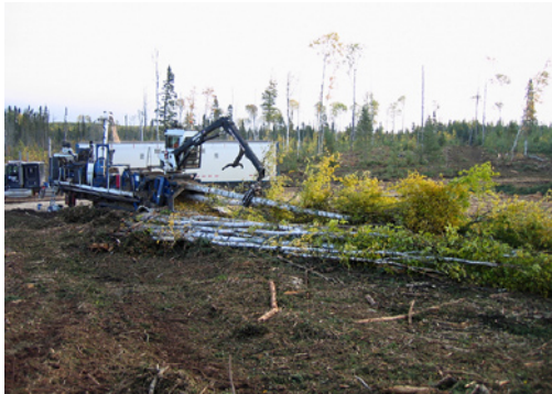
Figure 30. Whole tree chipping including a debarking unit starts to become more popular especially for high quality pulp and pellet production. © Dominik Röser, Metla
