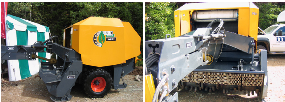
Figure 14. Bio Bales bundles for energy crops, the bales can be attached to a farm tractor. © Dominik Röser
