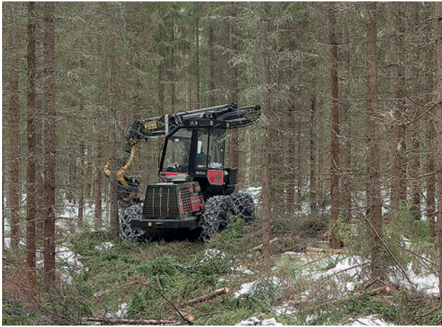
The Nordic cut-to-length (CTL) felling system and machinery is suited also to the conditions of first thinning without causing damages to the remaining trees on the site.
