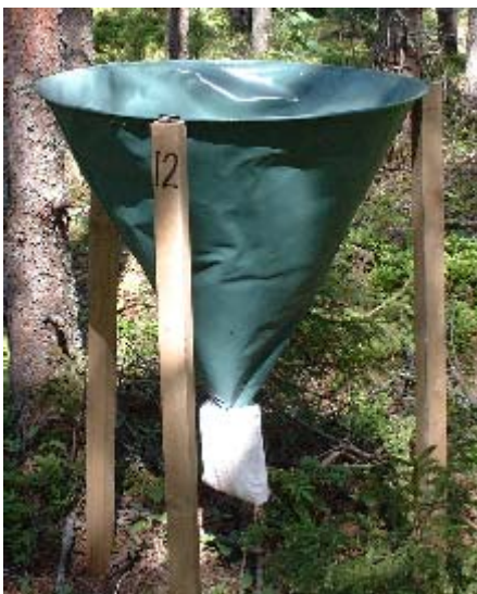
Figure 9. An example of a litterfall collector with an upper diameter of 80 cm (Photo: A. Ryyänen/Metla)
