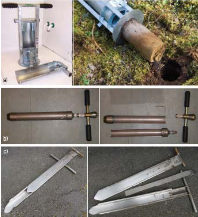
Figure 2. Examples of sampling devices for different soil types: soil corers for till soils (a) and sediment soils (b), and a peat sampler (c).
