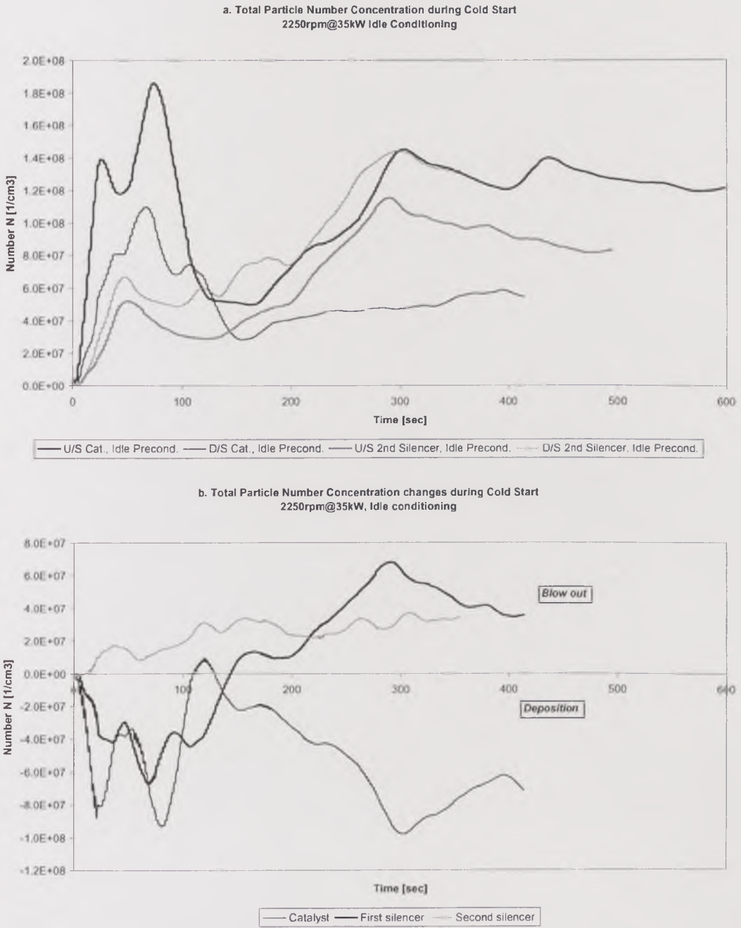
Figure 4.29. Total number and mass concentrations vs. time during cold start at high-load conditions after Idle preconditioning at various exhaust points. a) Particle number concentration.
