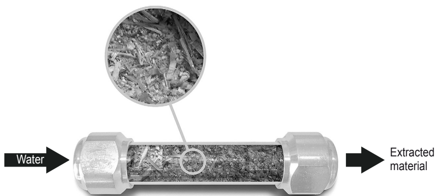
Figure 10. A 50 mL flow-through extraction vessel (Paper V).
