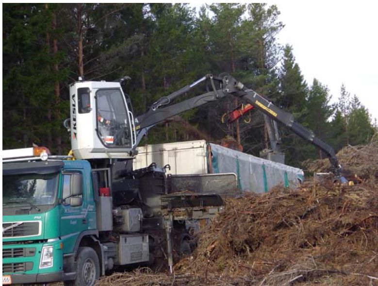
Figure 1 – Chipping pulpwood with the Kesla C 860 H hybrid chipper at the wood terminal in Joensuu (top) and chipping logging residues in Rauma (down).
