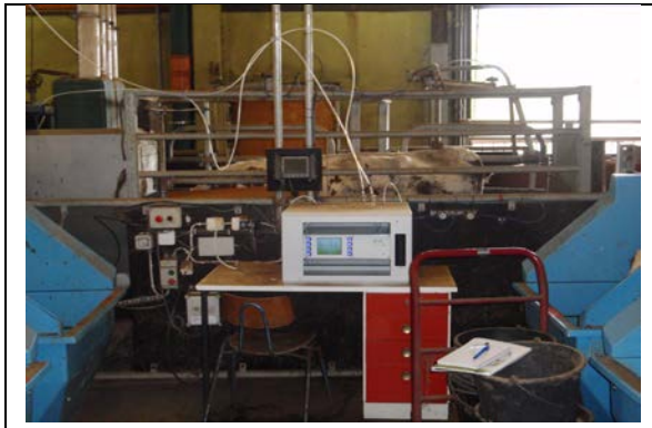
Figure 2. A two-point F10 Multi-gas analyzer set-up in operation with a cow in feeding kiosk getting her concentrate supplement while the gas sampling and measurements are made at the MTT Minkiö dairy barn.
