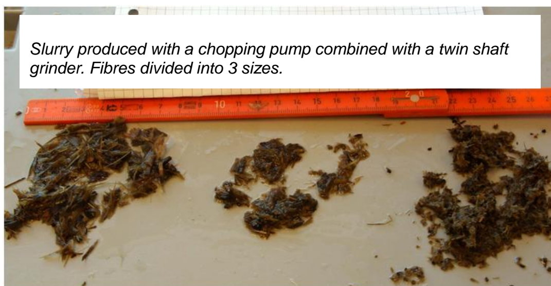
Figure 11.12. Particles from converted deep litter manure into a pumpable slurry.
