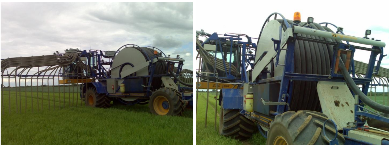
Figure 6.4.4. Umbilical distributor with boom and trailing hose applicators.
