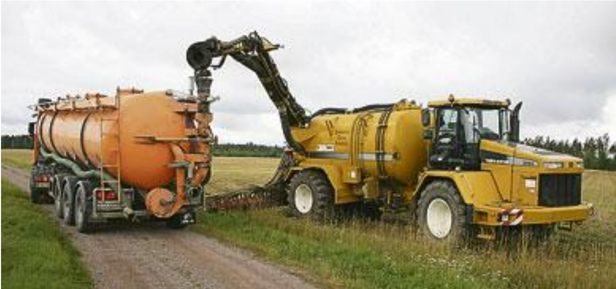
Figure 6.2.5. Pictures of slurry tanker with injection boom and nurse tank for transport.
