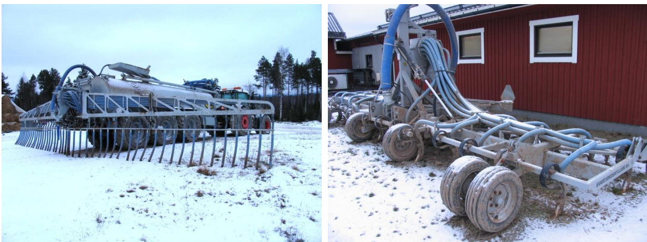
Figure 6.6.6. Picture of slurry spreading equipment used on farm 2: (A) the 16m boom with trailing hose applicators and HTC 20 m 3 tanker by Hill ( www.lkverkstad.se ) and (B) the 8 m wide arable soil slurry injector also by Hill (“Svartjordsmyllare”).
