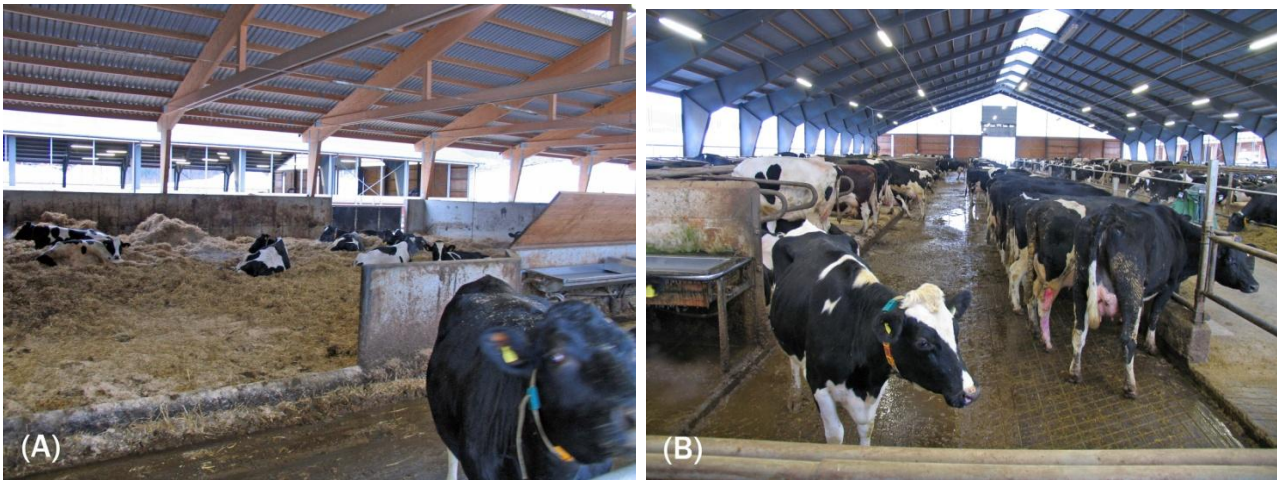
Figure 6.6.5. A) Loose deep-litter pens and passageway in the milking cow section of H1. B) One of the passageways in H2 with stalls on left and feeding access on the right towards centre drive-through and water trough in loafing areas in the front. The passageway is concrete with a textured pattern cut into surface to improve traction for cows.
