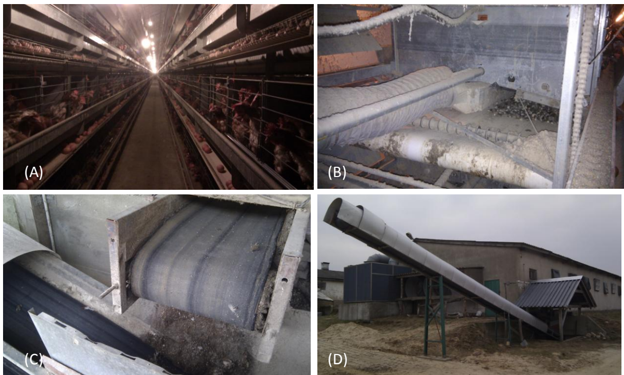
Figure 6.5.18. (A) Inside of one of the animal housing units, and (B-D) the manure removal system: B) view of the conveyor belt for mechanical manure removal from under the cages in use, C) manure transport from the indoor conveyor belt to outdoor conveyor belt, D) manure transport from outdoor conveyor belt to the mobile container.
