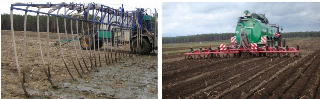
Figure 6.5.14. Manure spreading on Farm 3 and 4 with the usage of umbilical trailing hose applicator (Agrometer Pioneer) to the left and closed slot injection (Samson) to the right (source: POLDANOR).
