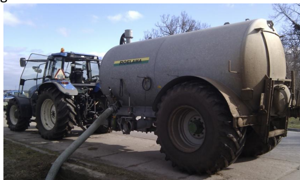
Figure 6.5.6. Slurry tank for pumping of the urine, household wastewater, rainwater and liquid manure from System 3 and as well for spreading.
