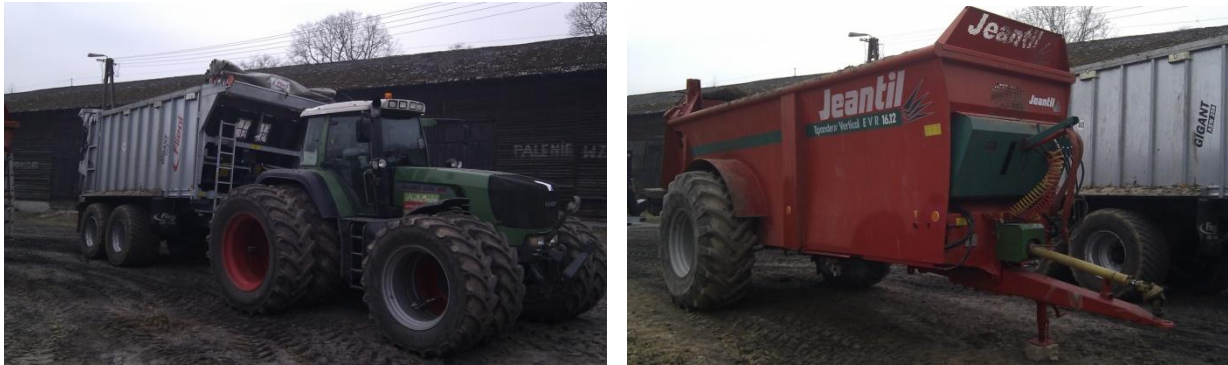
Figure 6.5.19. Broadcasters used for solid manure spreading: FLIEGL on the left and JEANTIL on the right.
