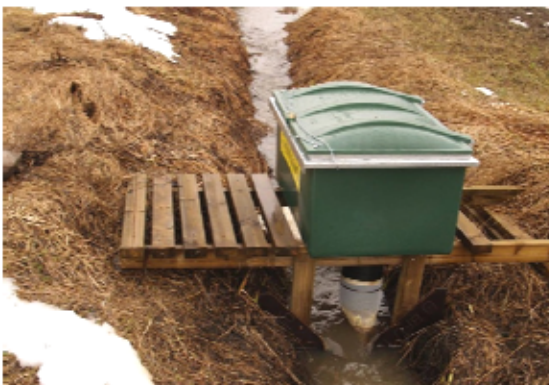
Figure 6. Upper graph: schematic figure of the Närvänen-type Ferix doser. The photographs show a smaller doser unit (left-hand) that is sized for relatively small ditches, and (right-hand) a larger unit that is equipped with two doser socks and a 600-litre storage compartment to ensure a high enough feed during peak flow. Photographs by Aaro Närvänen.
