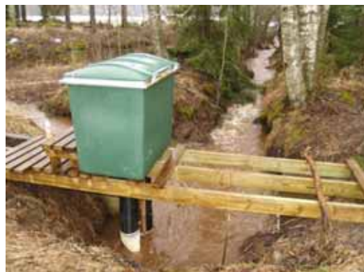
Figure 6. Upper graph: schematic figure of the Närvänen-type Ferix doser. The photographs show a smaller doser unit (left-hand) that is sized for relatively small ditches, and (right-hand) a larger unit that is equipped with two doser socks and a 600-litre storage compartment to ensure a high enough feed during peak flow. Photographs by Aaro Närvänen.
