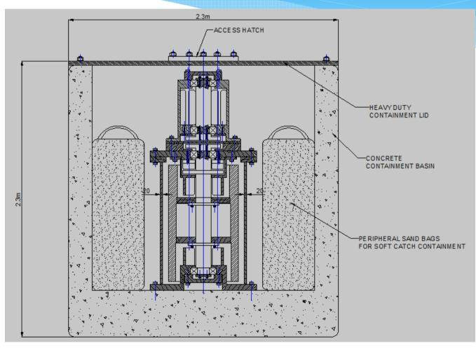
**Containment Option Two: Concrete Basin with Sand Bag Soft-Catch**
