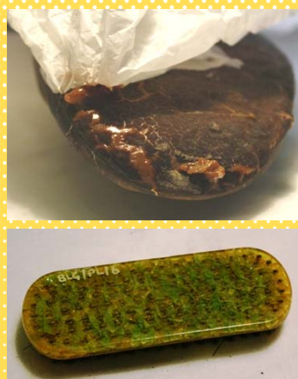
Figure 3. Top, plimsoll showing area of sole adhered to acid free tissue. Bottom, deteriorating cellulose nitrate brush.
