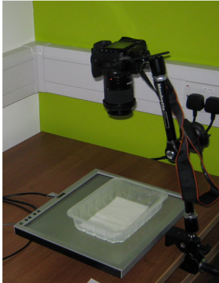
Figure 7: The makeshift polariscope used to make the polarised light stress patterns, comprising an LCD monitor and a CCD camera with a linear polarising filter at 90^\circ to the polarisation of the light coming from the LCD. The item to be inspected is placed between the two.
