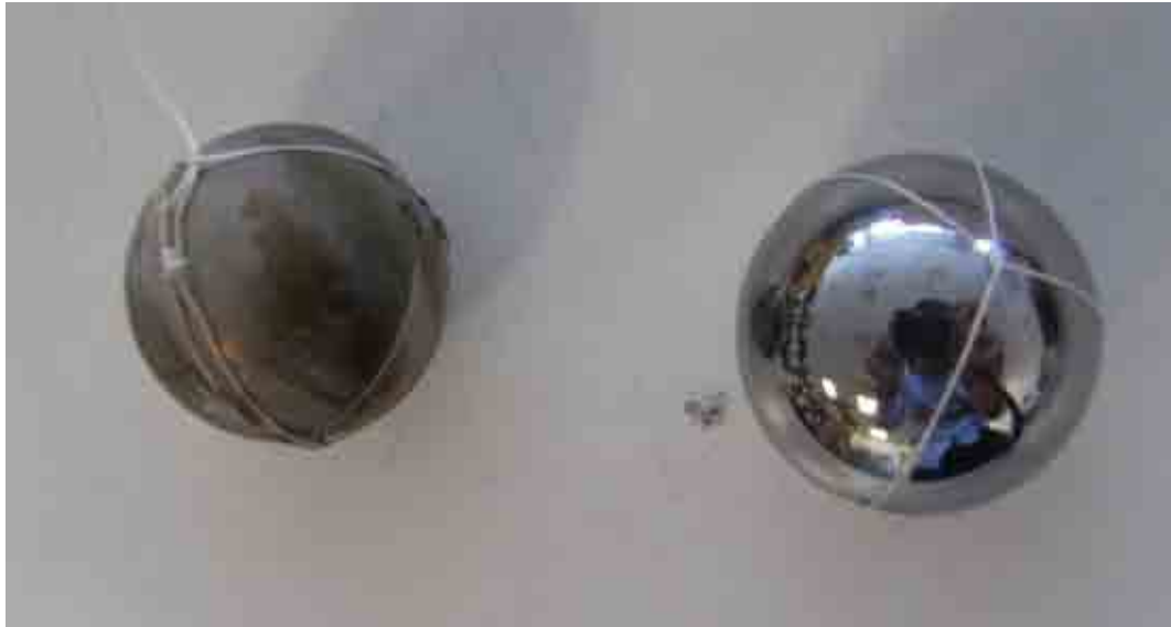
FIG. 5.10. Corrosion performance compared after approximately equal immersion time. Left, cobalt-binder tungsten carbide sphere. Right, nickel-binder tungsten carbide sphere.
