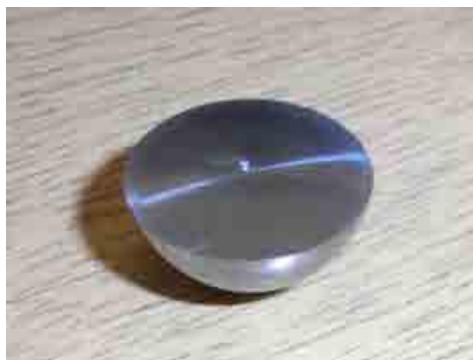
FIG. 5.8. Cut hemisphere of 20 mm (A) TC/Co sphere.
