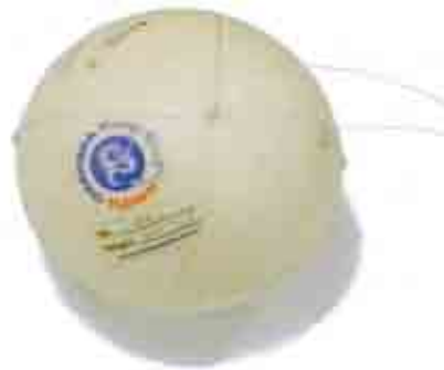
FIG. 7.17. Air-filled ceramic shell.
