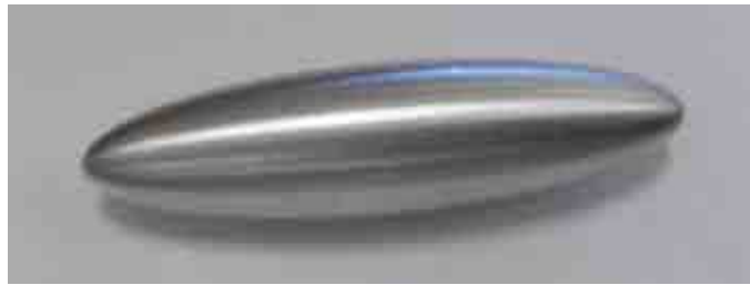
FIG.7.30. Machined aluminium prolate spheroid.
