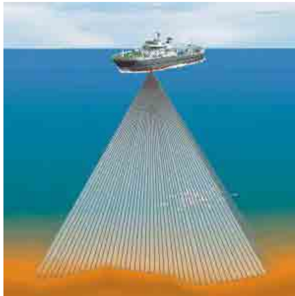
FIG. 1.2. Scientific multibeam echo sounder, Simrad ME70 (from www.simrad.com ).
