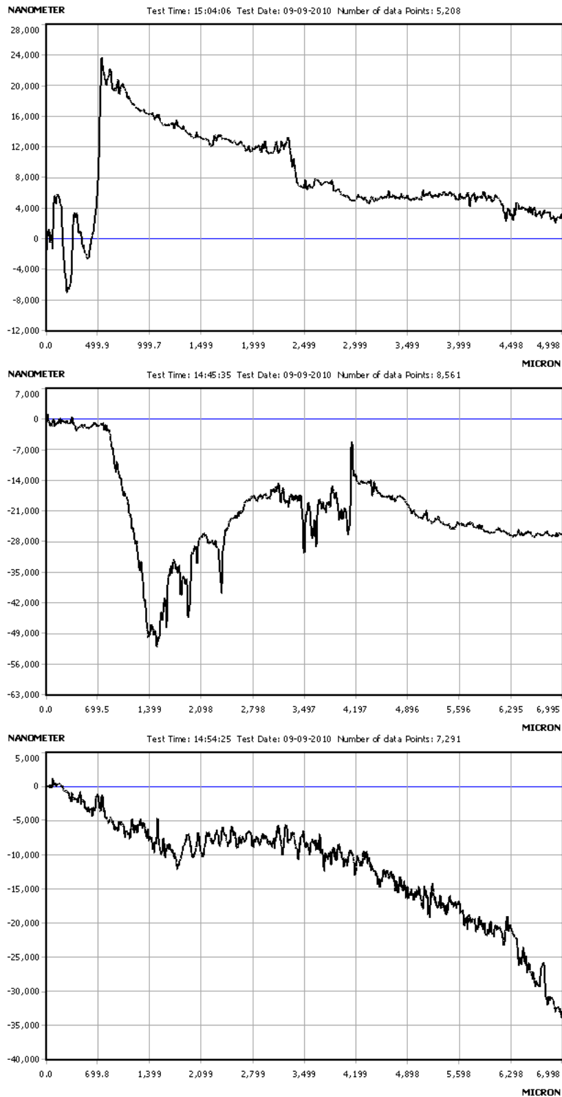
Figure 43 – Surface Roughness profiles, PP synthetic ice counter-face wear tracks for (a) AISI316 Untreated, (b) AISI 316 Carburised, (c) AISI 316 Nitrided following sliding simulation testing
