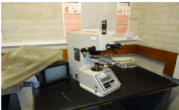
Figure 8 - (a) Matusoyo Micro-Hardness indenter, (b) Knoop indent
