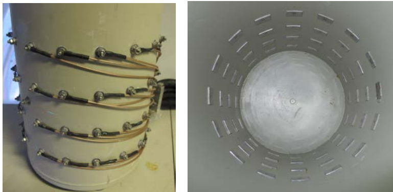
Figure 5.7. An overview of the external and internal electrode arrangements of the circular array ERT vessel
