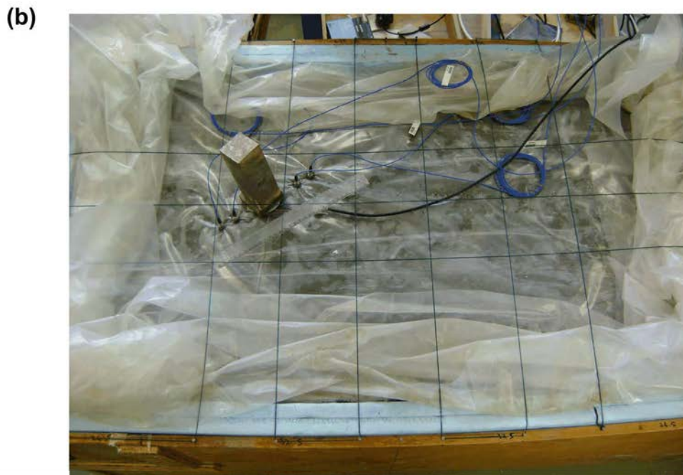
Figure 6.12: (a) Final layout of test programme where no. 1 to 7 were good quality columns, no. 8 defective column and no. 9 large diameter column, and (b) photograph of the Oxford clay model covered with cling film and plastic to avoid water desiccation.
