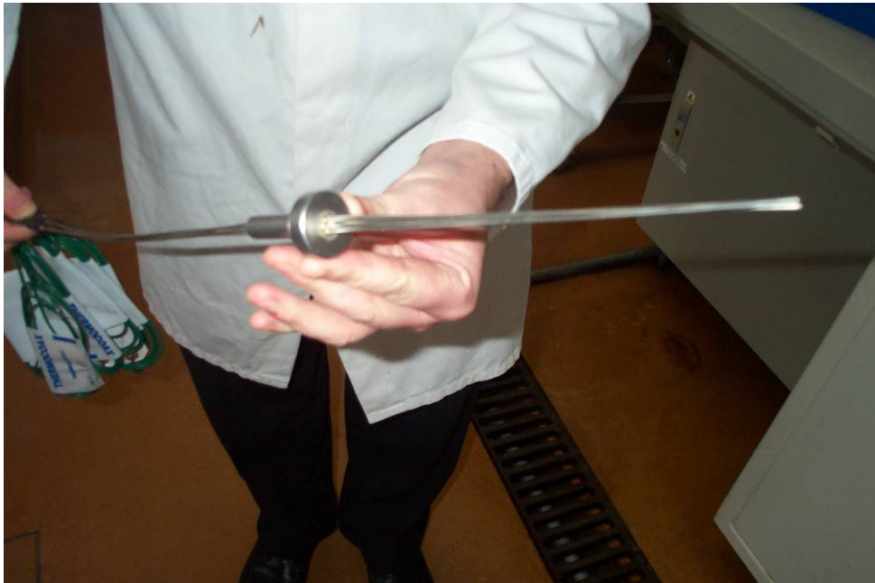
Figure 3-4. Thermocouple feed-through used for temperature distribution studies
