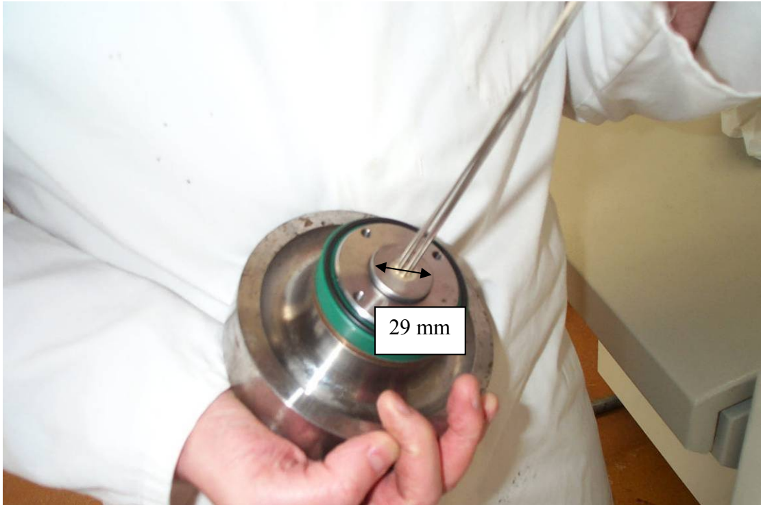
Figure 3-11. Final feed-through assembly used for experiments in stage 3. The feed-through is pictured in place on the top closure of the vessel. A securing plate screwed to the bottom of the closure completed the installation.
