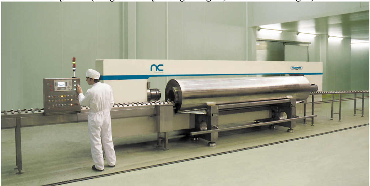
Figure 1-4. A horizontal batch high pressure processing vessel (covers removed) from nc Hyperbaric (image courtesy of Carole Tonello, nc Hyperbaric)
