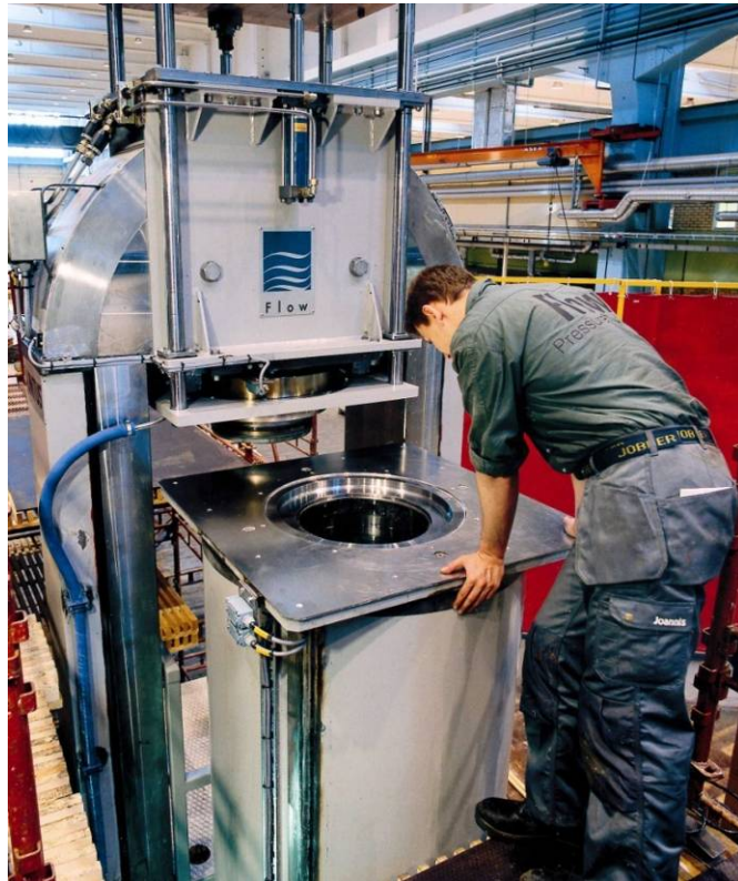
Figure 1-3. A vertical batch high pressure processing vessel from Avure Pressure Systems (image courtesy of Nigel Rogers, Avure Technologies)
