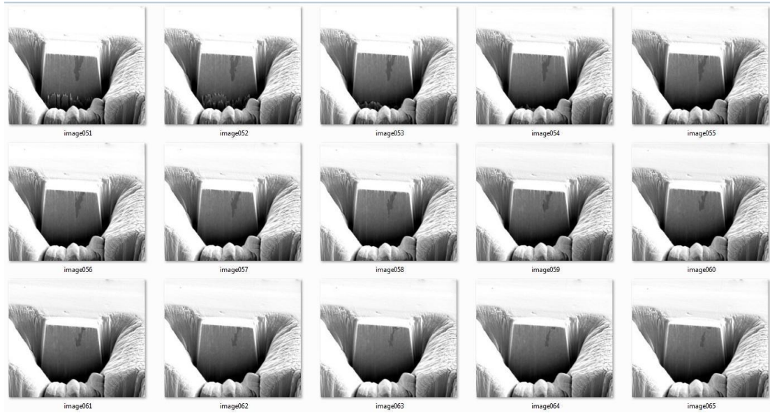
Figure 19: Successive FIB slices through rail steel showing the variation in inclusion deformation.
