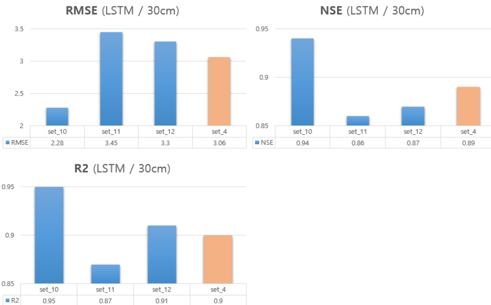
Figure 52 RMSE, NSE, and R2 values of LSTM model predictions at a depth of 30 cm
