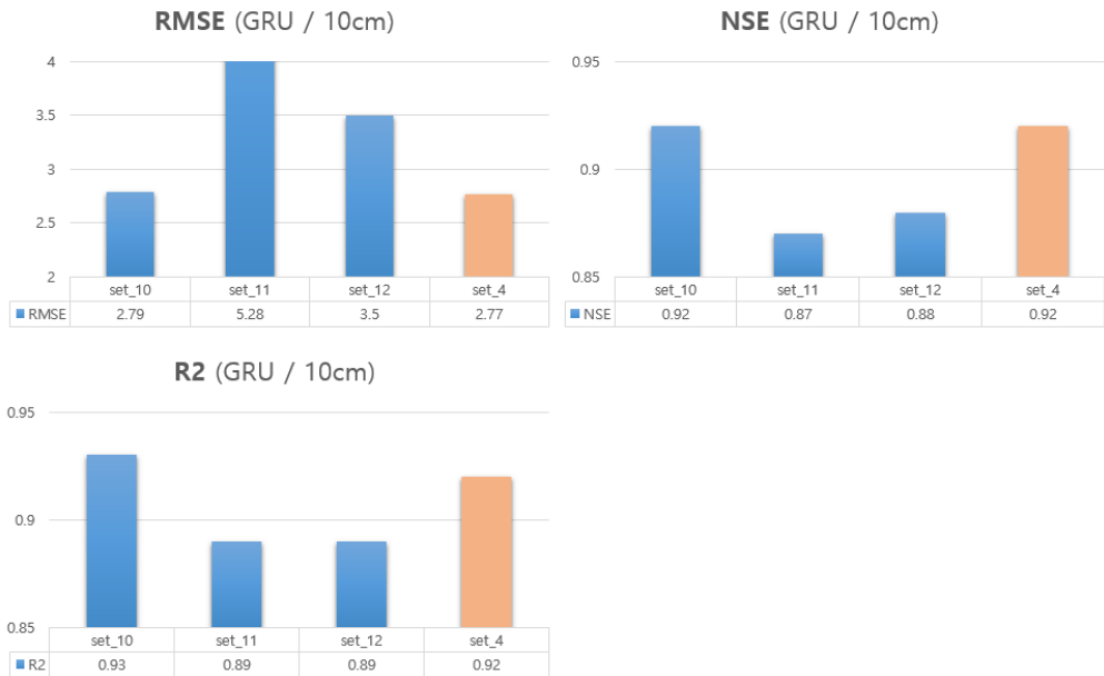
Figure 47 RMSE, NSE, and R2 values of GRU model predictions at a depth of 10 cm
