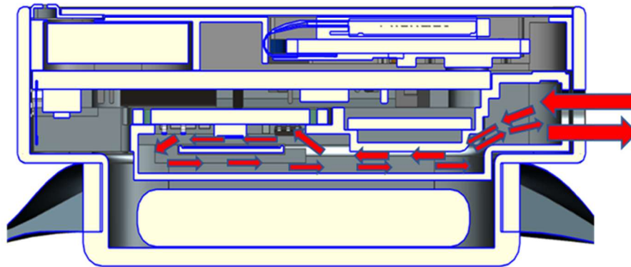
Figure 34. Teardown and Gas path design (a) Teardown of wearable gas sensor (b) Gas path design
