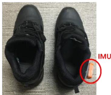
Figure 5.7: Foot mounted IMU used in experiments
