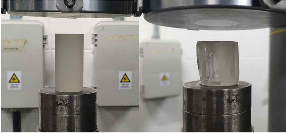
Fig. 3.4 UCS test with 3D printer material (VeroClear): (a) 3D printed specimen before testing, (b) 3D printed specimen after testing
