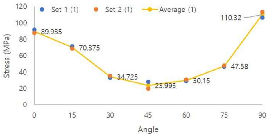
Fig. 4.5 3D printed specimen UCS test results, MTS (0.0067 mm/s)
