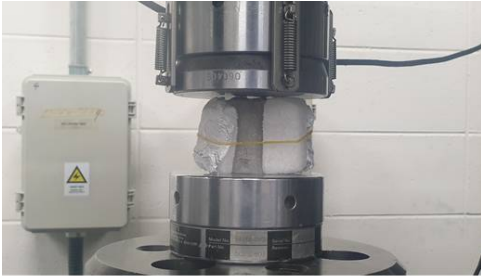
Fig. 3.5 UCS test for a VeroClear 3D printed specimen with dry ice attached
