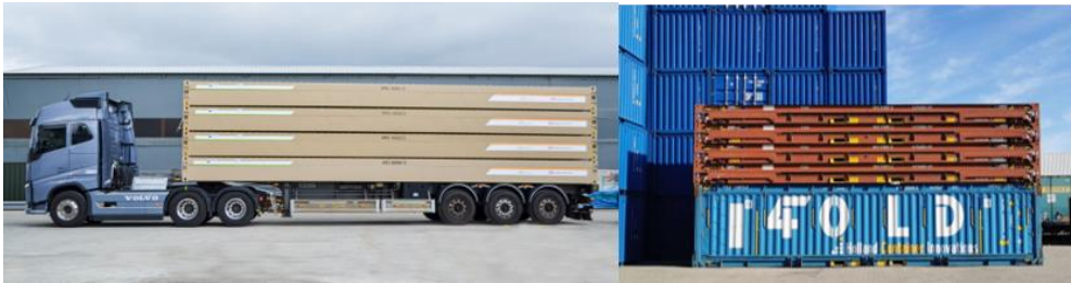
Figure 1.1: Foldable containers currently developed(left: KRRRI[2]; right: HCI[5])
