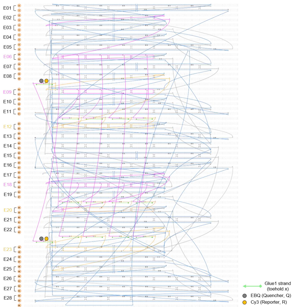
Figure A8. caDNAno blueprint of SQ H2 (3-pair) with two reporters and quenchers.
