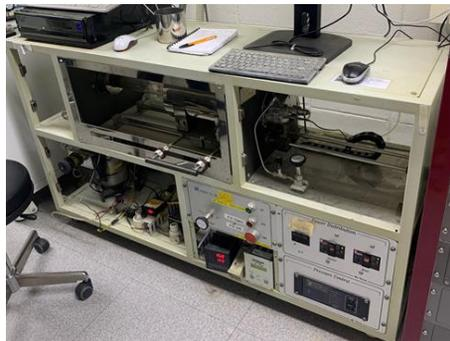
**Figure 3.6** Vacuum furnace: thin film samples were subjected to vacuum annealed (< 0.0013 Pa) for surface diffusion.
