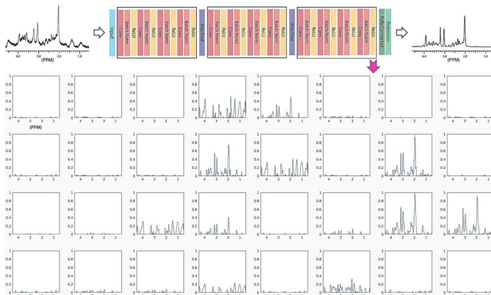
Figure 2-15. The activations of the twelfth ReLU layer for all of the 32 channels.
