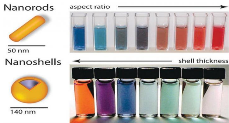
Figure 1.5 Optical properties of gold nanoparticles with different shapes and sizes. Gold nanorods (top), and silica-gold core-shell nanoparticles (bottom).
