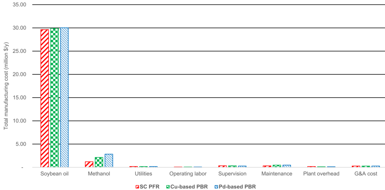
Figure 9 The proportions of subitems in the total manufacturing cost for each biodiesel production process.
