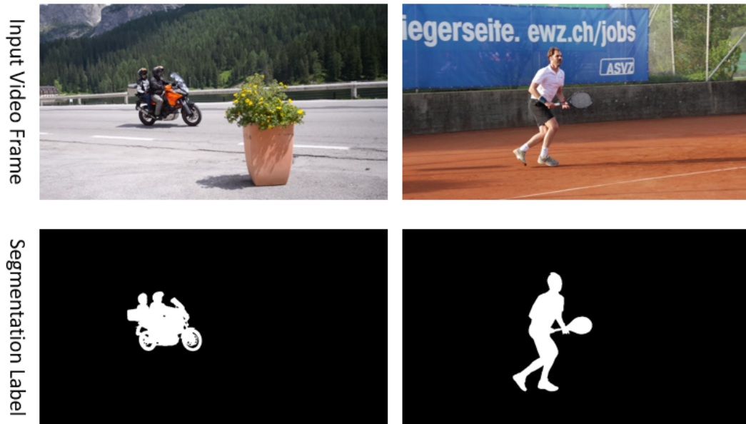
Figure 1.6: An example of a popular dataset used for video segmentation. [1] The input frame. [2] The corresponding segmentation ground truth map.
