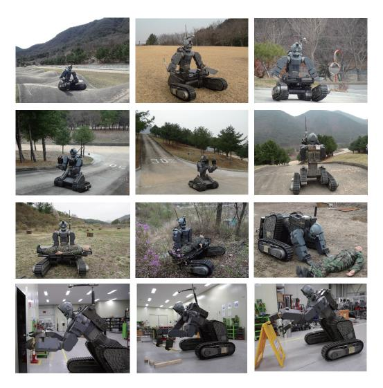
Figure 4.3: Various poses of the rescue robot, Hurcules: drive and task execution postures.
